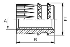
Female thread A = M2,5 Length B = 4.0 Max outer diameter E = 4.0 Number of cramping feathers = 1
